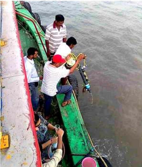
Water-sampler being deployed during cruise
