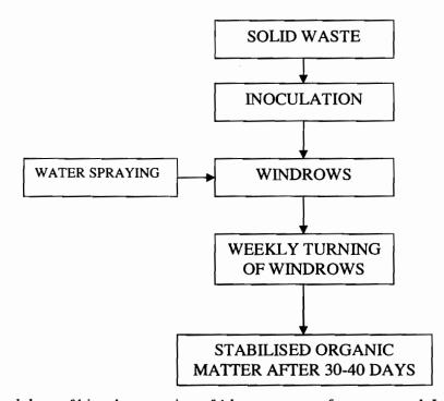
Total dose of bioculum consists of 1 kg per tonne of waste treated. It is given in three stages i.e. in the beginning, before first turning and before second turning. Total water requirement during complete process is about 200 lit per tonne of waste treated.
